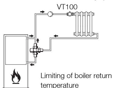
Limiting of boiler return temperature
