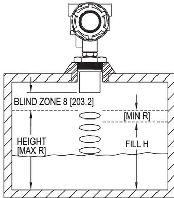
Figure 8: Target calibration
