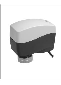
AMI 140 is 2 point 3 wires actuator used with AB-QM (DN 10-32) and VZ, VZL, VRBZ valves. The actuator can be used with fan coil units, induction units, small re-heaters, re-coolers and zone applications in which hot/cold water is the controlled medium. The actuator provides with factory default setting (actuators spindle fully stem up):
