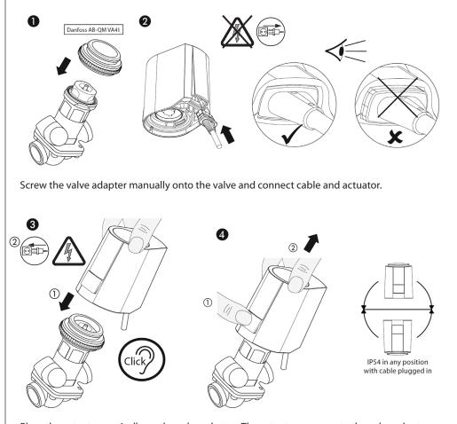
Place the actuator vertically on the valve adapter. The actuator snaps onto the valve adapter with a "click" when pressed down vertically by hand. Do not apply power until the actuator is mounted on the valve.
