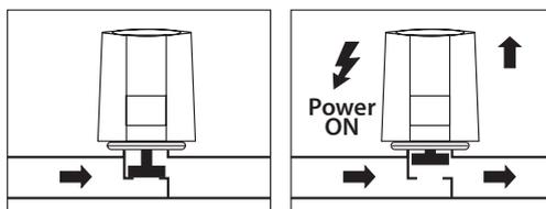
Function display for NC versions extends proportionally with actuator opening from 0 mm to 5-6 mm.
